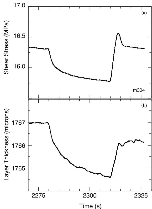
**Figure 8.** (a) A 30-s SHS test from Figure 3a is shown with (b) corresponding layer thickness change. Compaction occurs during the hold as shear stress relaxation occurs. When loading resumes, the layer dilates to accommodate displacement.
