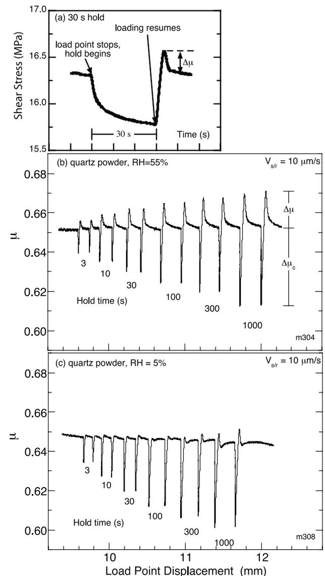
**Figure 3.** SHS tests for quartz powder. (a) Typical 30 s hold shows frictional creep when load point stops and stress peak when loading resumes. (b) Typical set of SHS tests performed at 55% RH illustrate frictional creep ( $\Delta\mu_c$ ) and frictional healing ( $\Delta\mu$ ). (c) Under dry conditions, with the same displacement history shown for panel b, healing is negligible.
