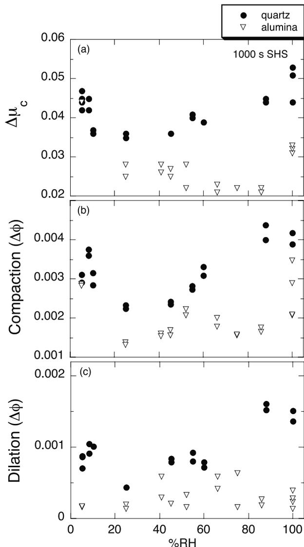
**Figure 11.** (a)  $\Delta\mu_c$ , (b) compaction, and (c) dilation all vary with RH for both alumina and quartz. The largest values for creep, compaction and dilation occur at very low and very high RH.
