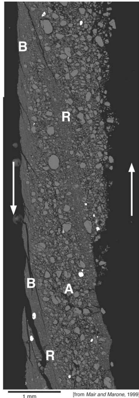
**Figure 1.** Backscattered electron micrograph of a granular layer after 20 mm of left-lateral shear at  $\sigma_n = 50$  MPa [Mair and Marone, 1999]. Areas of intense comminution are interpreted as boundary (B) and Riedel (R) shears. These zones are surrounded by relatively undisturbed regions (A), where little slip occurs.
