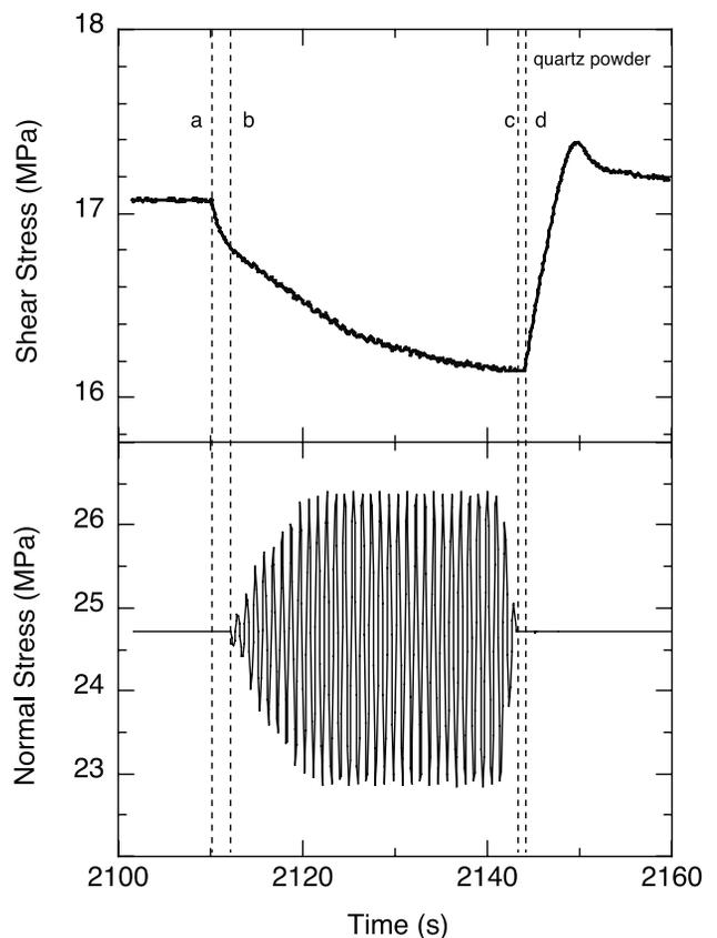
**Figure 12.** Shear stress and normal stress versus time for a quartz-powder SHS test with normal stress oscillations. Fiducial lines mark where the load point stops (line a), oscillations begin (line b), oscillations stop (line c), and shear loading resumes (line d). Note that oscillation amplitude increases gradually over roughly a 5-s interval.
