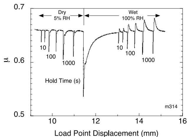
**Figure 4.** Humidity step test showing the effect of adding water to a low RH experiment. Healing is negligible under dry conditions, but after water is added distinct frictional peaks and time-dependent healing are observed.
