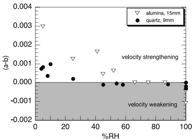
**Figure 16.** Friction exhibits velocity strengthening behavior at low humidity for both quartz and alumina powders. A transition to velocity neutral or velocity weakening behavior occurs at  $\approx 35\%$  RH for quartz and  $\approx 65\%$  RH for alumina. Alumina exhibits a greater humidity dependence of  $(a-b)$  than quartz.
