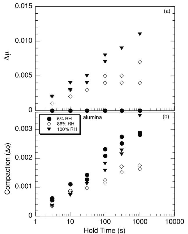
**Figure 10.** (a) Three representative sets of healing data for alumina powder. Healing is negligible at 5% RH, and increases with increasing RH. (b) Compaction proceeds linearly with log hold time and is independent of RH.
