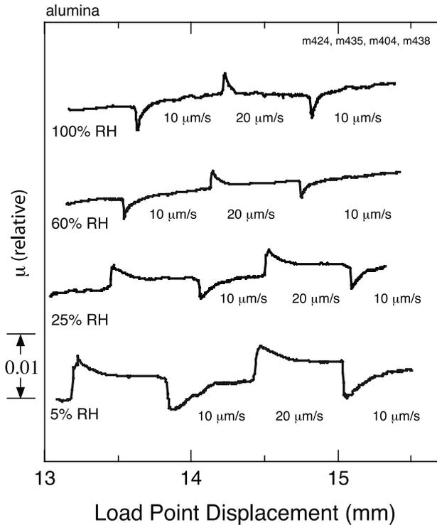
**Figure 15.** Four sets of alumina powder velocity-stepping tests performed at different values of RH. Friction data are offset vertically for clarity. The low humidity tests demonstrate velocity strengthening. At 14–15 mm displacement, alumina powder becomes velocity neutral at RH >60% and velocity weakening at 100% RH.
