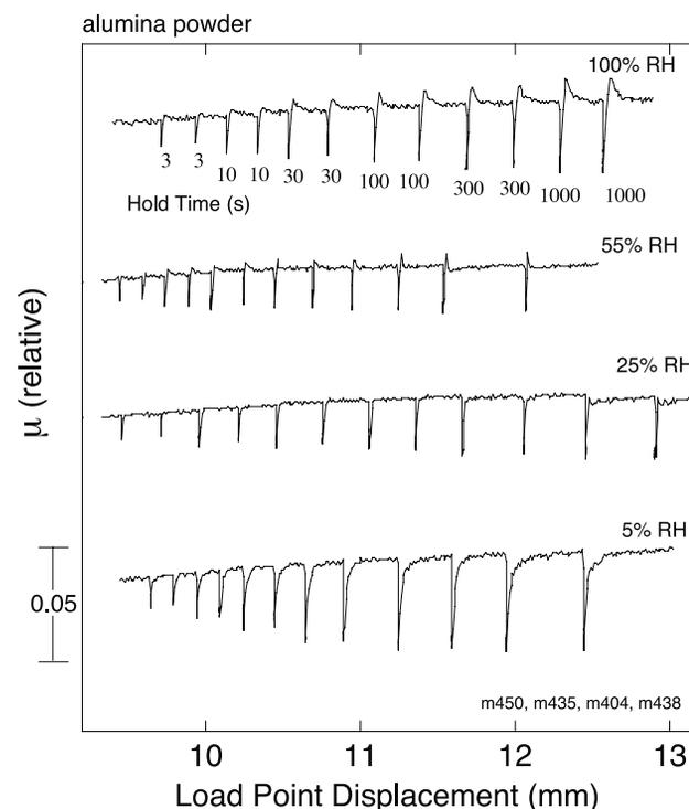
**Figure 6.** Data from four experiments on alumina powder performed at different values of RH. The same sequence of hold times, labeled on the 100% RH test, were used in each experiment. Friction is offset vertically for clarity. The low humidity tests exhibit little healing. Frictional peaks become measurable above 50% RH. The evolution distance needed to reach steady state sliding after a hold is negligible for the intermediate RH cases.
