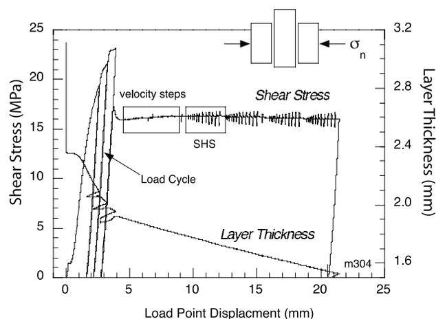
**Figure 2.** Shear stress and layer thickness history for an entire experiment. Gouge layers are subject to three shear load cycles at high normal stress (40 MPa) to create fresh surface area before velocity stepping tests and SHS tests are carried out at normal stress 25 MPa. Layer thickness decreases throughout the experiment due to comminution and geometric thinning. Superimposed upon this thinning trend are layer thickness perturbations associated with velocity steps and SHS.
