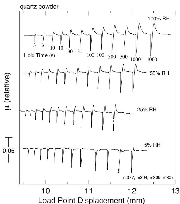
**Figure 5.** Data from four experiments on quartz powder performed at different values of RH. The same sequence of hold times, labeled on the 100% RH test, were used in each experiment. Friction is offset vertically for clarity. The low humidity tests exhibit little healing. Healing rates increase with humidity and approach a constant value above 55%. The evolution distance needed to reach steady state sliding after a hold increases with RH.
