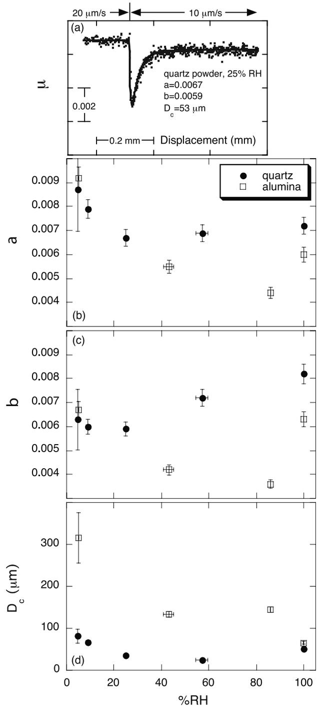
**Figure 17.** The velocity dependence of quartz and alumina powder was modeled using the Dieterich [1978, 1979] formulation of the rate- and state-friction law. (a) Raw data and model fit for a 20–10 mm/s velocity step shown for quartz powder at 55% RH. (b) The model parameter  $a$  is plotted versus RH for alumina and quartz samples. (c) The model parameter  $b$  is plotted versus RH at the same scale as Figure 17b. (d) The parameter  $D_c$ , the evolution distance, is plotted versus RH.
