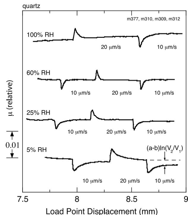
**Figure 14.** Four sets of quartz powder velocity-stepping tests performed at different values of RH. Friction data are offset vertically for clarity. The low humidity tests demonstrate velocity strengthening. At 8.5–9 mm displacement, quartz powder becomes velocity neutral at 60% RH and velocity weakening at 100% RH.
