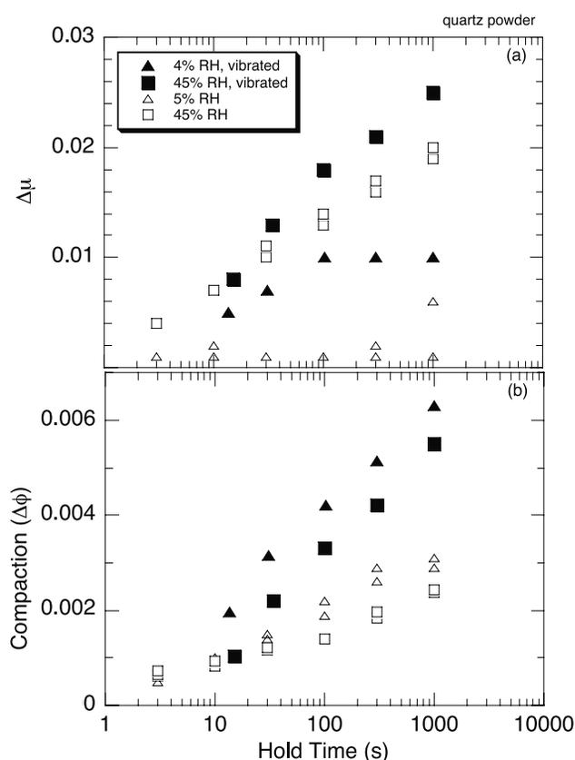
**Figure 13.** (a) Healing versus hold time for vibrated and constant normal stress SHS tests (quartz powder). Data from vibrated tests show greater healing than constant normal stress tests at a given humidity. In the dry tests, vibration enhanced healing becomes constant for hold times greater than 100 s. (b) Compaction during normal stress vibration tests are approximately double those of constant normal stress tests.
