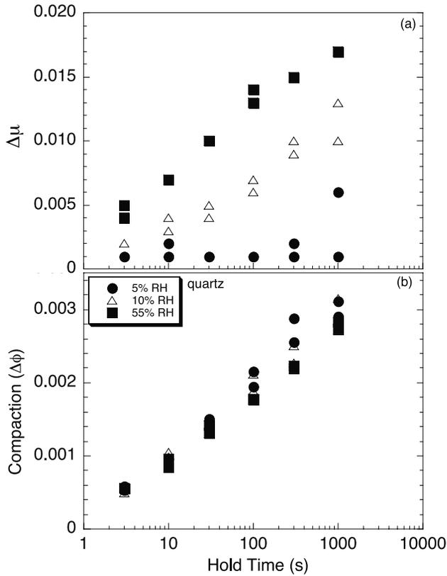
**Figure 9.** (a) Three representative sets of healing data for quartz powder. Healing is negligible at 5% RH, and increases with increasing RH. (b) Compaction proceeds linearly with log hold time and is independent of RH. Compaction is defined as change in layer thickness during the hold divided by layer thickness before the hold.
