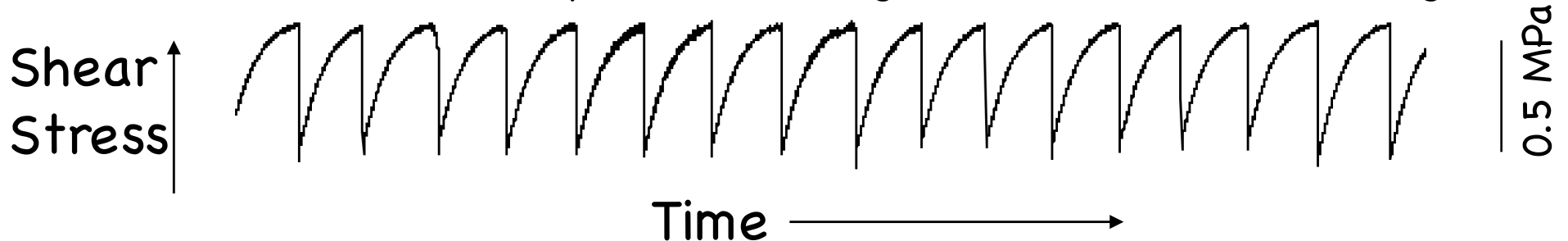
Stick-slip failure during shear at constant loading rate
