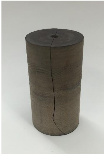
Figure 1. Fractured sample and the typical pressure change during HF experiment.
