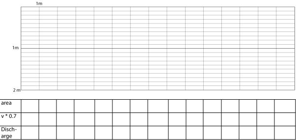
Note: you take 70% of the surface velocity in order to approximate the average velocity from the surface to the bed of the stream (where the velocity diminishes).
